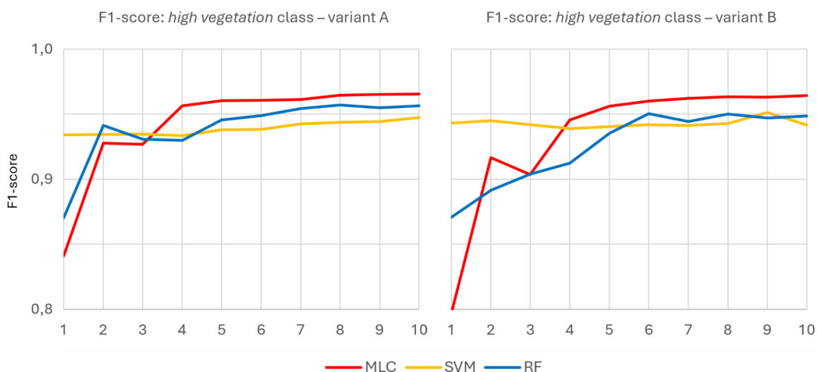
Fig. 7. Diagram of F1-score values for the high vegetation class using individual ML algorithms depending on the training sample size, for variants A and B.
